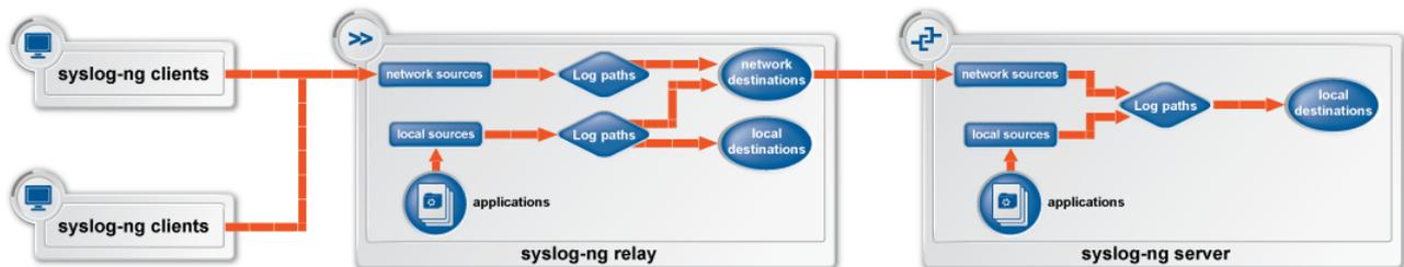
Figure 2.3. Relay-mode operation
