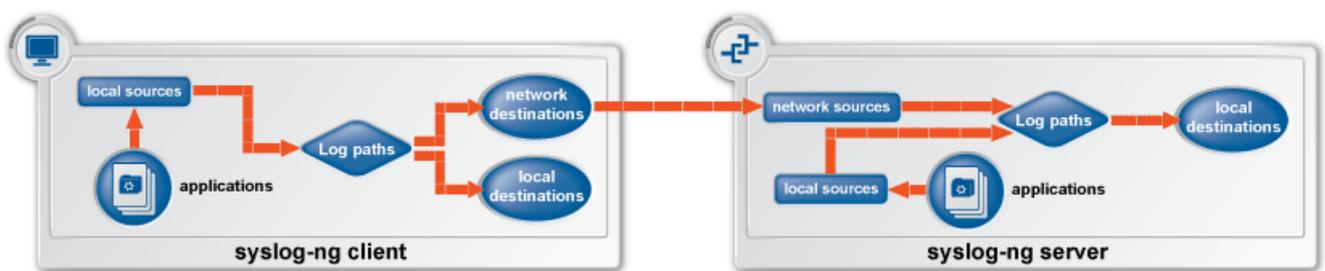
Figure 2.2. Client-mode operation
